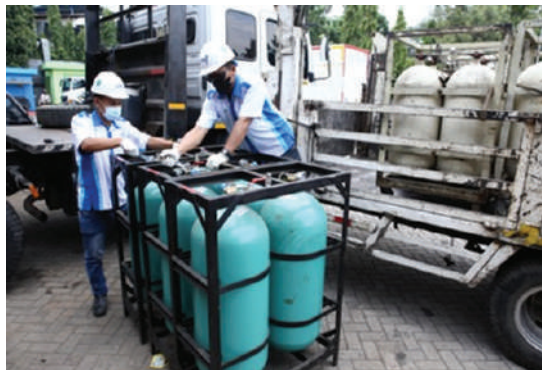
GTM Retail Cradle Capacity : 40 sm 3
