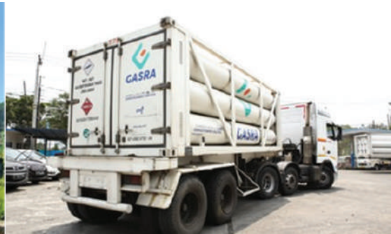
GTM Industri GTM : 20 Feet Capacity : 2.800 sm 3
