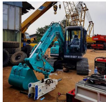
Excavator Kobelco SK75P-8 (Bucket + Breaker)
