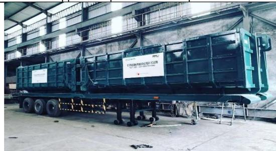
Semi-Trailer Arm Roll Box for Hazardous Material
