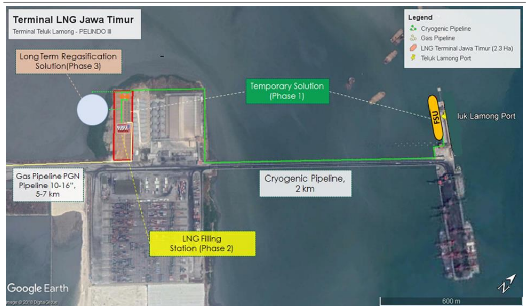
Figure 18: LNG Infrastructure in Teluk Lamong
